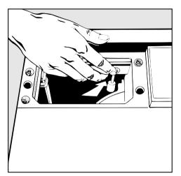
Close the water inlet port above the condensed water container with the bottom part of the rubber plug. The plug must face towards the interior of the machine so that the condensed water container can easily be inserted.
